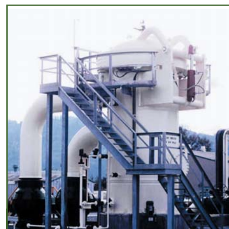
This Absolute Separator is installed in a metering station in Canada. Its 2500 mm ID housing utilises a full diameter, quick-opening closure.
