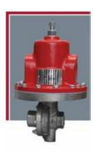
The Mark 63 is designed to maintain a constant differential between the pressure on the discharge side of the regulator and the signal pressure loaded on the diaphragm. The Mark 64 provides the same flow capacity but with less offset. It features a larger effective diaphragm area for greater sensitivity.
