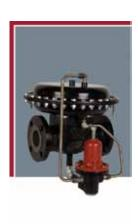
The Jordan Mark 687 is a piloted soft seat regulator for critical pressure reducing applications. It uses balance plug trim with the action of a pilot valve to create a faster, more accurate (meaning less droop as your flows increase) response.
