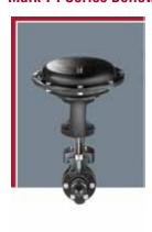
The Mark 74 provides exceptional bellows life with a valve stroke that is just a fraction of that of other rising stem valves. This means Jordan Valve can use a smaller formed bellows that has minimal movement during operation.
