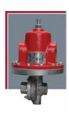
The Mark 53 is designed to maintain inlet pressure at a set differential pressure over the signal pressure loaded on the diaphragm. The Mark 54 provides the same flow capacity as the Mark 53 but with less offset in controlled pressure due to a larger diaphragm.
