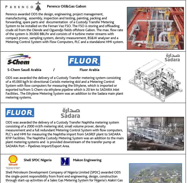
Field. The scope of supply comprised of a 2x100% 12" 600# orifice sales gas metering skid and a complete analyser package with redundant analysers such as field mounted process gas chromatographs and dew point analysers. A Metering Control System with redundant Supervisory Computers was included to visualise all the field signals and act as overall control system.
